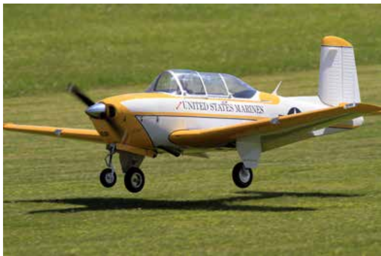
The T-34B, built by Mike Barbee and flown by Will Barringer in Team Scale, coming in for a landing. The 155-inch wingspan model is completely detailed with fiberglass construction.
