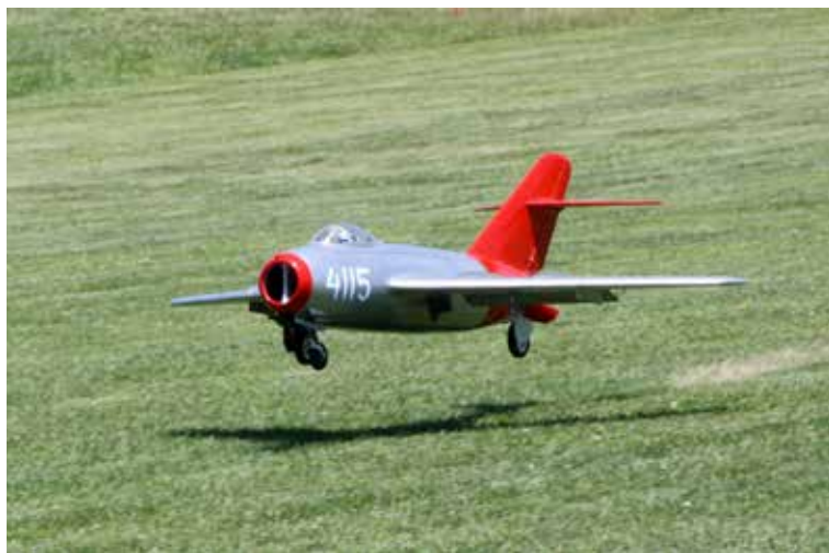
Terry Nitsch's BVM EDF MIG 15 entered in Fun Scale Open features air brakes and a drop tank, as well as an electric-ducted fan and a DX18 Spektrum radio system.
