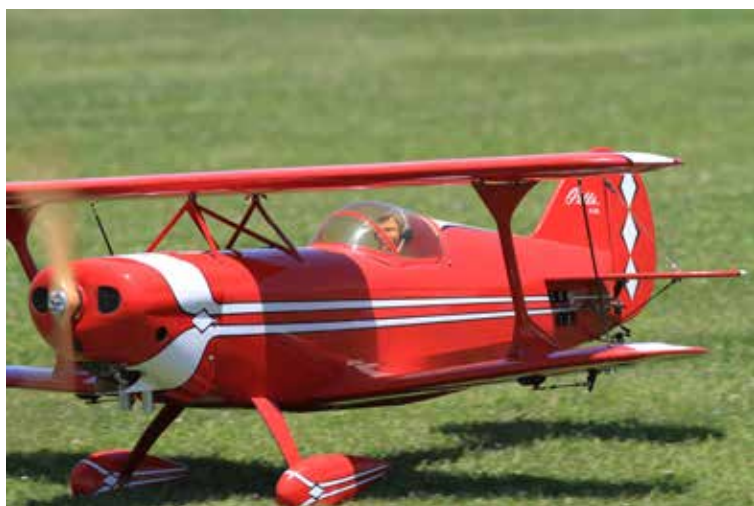
The Pitts S2B, entered in Fun Scale Open by Tim Lovett from Texas, has a wingspan of 68 inches and is flown with an Airtronics SG10 radio system powered by a DLE 55.
