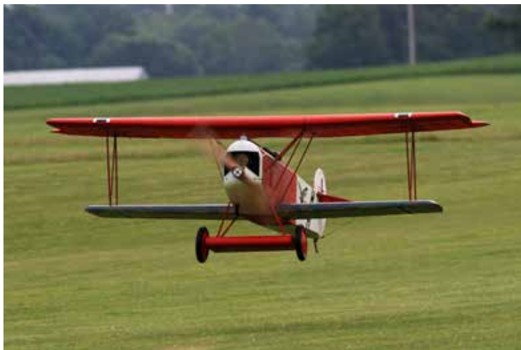
Joe Vermillion's Fokker D.VII 1/3 scale on his way to winning Fun Scale Novice. The large WWI model has a G-62 on belt drive for power. The kit is by Balsa USA.
