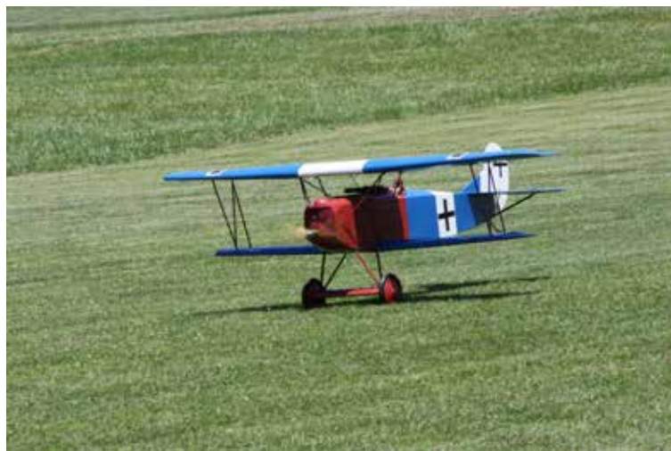
Dale Arvin's Fokker DVII on a take-off roll on some very smooth grass. The 1/4-scale model is powered by a Laser 240 V twin controlled with a Futaba radio system. It was built from a kit by Balsa USA.
