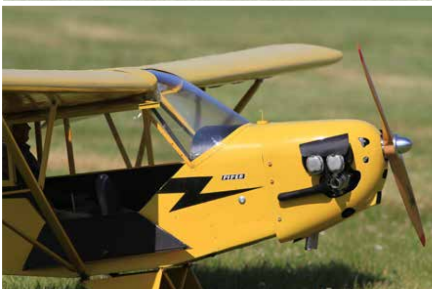
Cowl and engine details on David Folk's J-3 Cub, powered by a G-62 engine.
