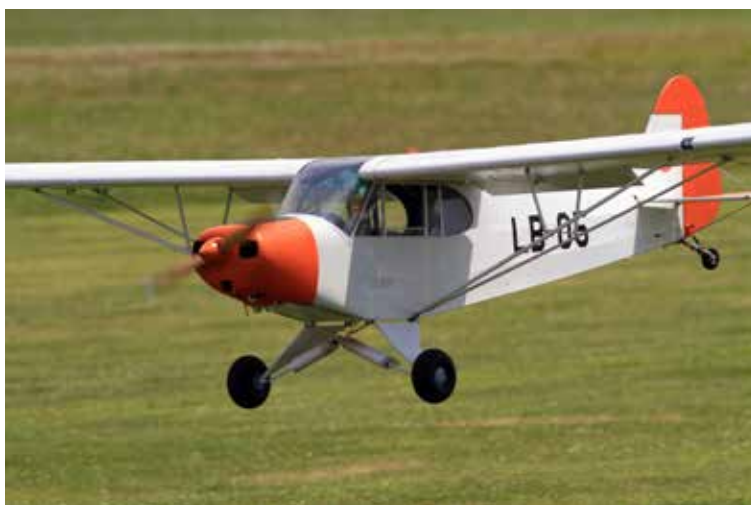
Ted Roman's Balsa USA Super Cub in Belgian Air Force colors won in Open Scale. The big 1/3-scale model is powered by a DLE .55 and controlled by a Futaba T14SG radio system.
