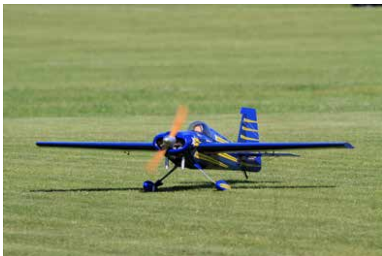
The Laser 200 by Joe Grubb, father of Adam Grubb, is built from a Lanier kit with a wingspan of 102 inches and power from a 3W 70cc gas engine.
