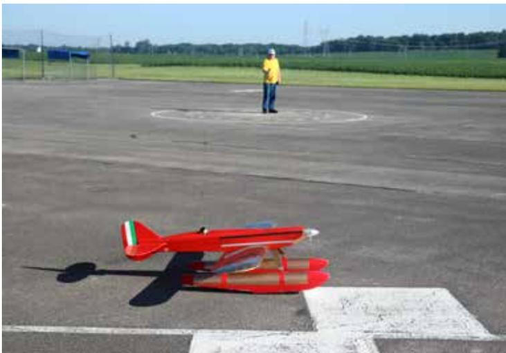
Grant Hiestand's Macchi 72 is not floating. The wheels in the floats are just high enough to allow the model to roll, take off, and land.
