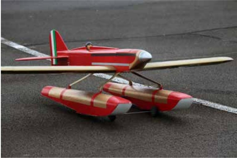
The foam wheels are visible from the front and provided good ground handling during takeoff, landing, and taxiing.
