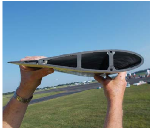
The inside of the wing of Dorin's composite plane.
