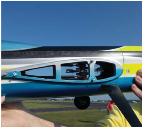
Dorin's composite plane's control hookups.
