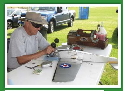
Burt Brokaw's MO-1 required some major field maintenance to replace a faulty check valve in the fuel system.
