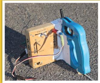
Pete Klepsic uses a three-line system for the throttle on his Profile B-25, but also has Clancy Arnold down-the-line electronic controls for the flaps, turret, and bomb drop.
