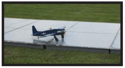
Profile Navy Carrier is flown with simpler models with profile fuselages and restricted fuel systems. This is the most popular Navy Carrier event. Shown is Bob Hawk's F8F Bearcat.
