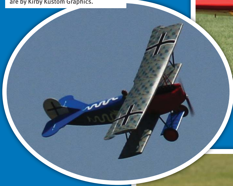
The Fokker D.VII by Michael Callahon showing off the lozenge camouflage on its top wing. It's powered by a U.S. Engines .41 gas motor. The snake logos are by Kirby Kustom Graphics.
