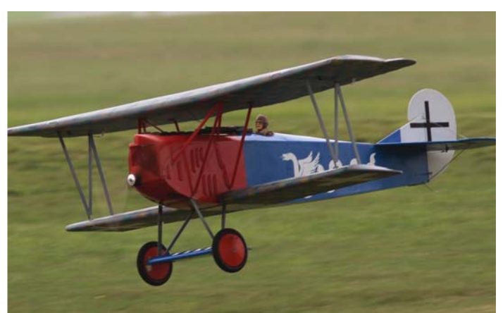
This Fokker D.VII is by Michael Callahan of South Lebanon OH. It's finished with Latex paint and the lozenge paint is hand painted.
