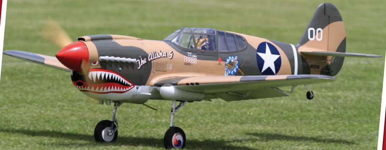
The Alisha G P-40 is a modified Top Flite ARF by Dan Landis. It's powered by a DA-50 engine using a Spektrum 10X radio.
