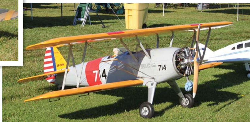
Mike Barbee's Stearman Fun Scale entry was powered by an Evolution gas radial engine.
