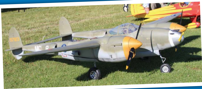
Mike Fearing's Zivko P-38 had a 115-inch wingspan and was powered by two DL-50 engines.
