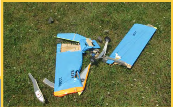
The most spectacular event of the day involved Mike Anderson's Skyray. The fuselage failed during high-speed flying, followed by the wing failing in positive loading, and the virtual disintegration of the aircraft in midair.
