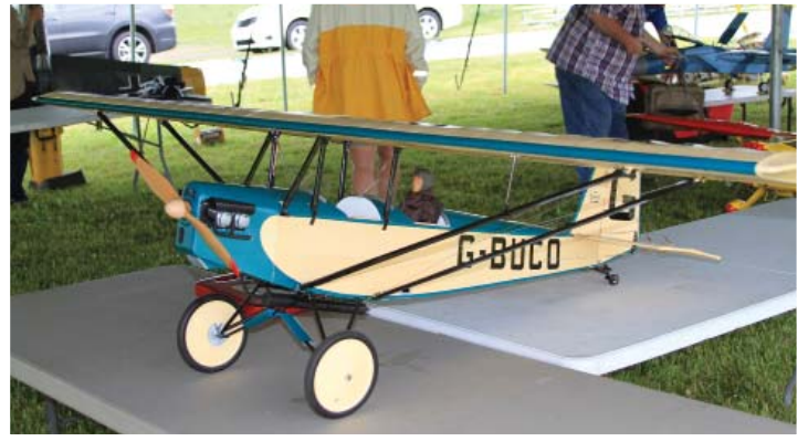
A scratch-built Pietenpol Air Camper built at 1/4 scale and very well detailed.
