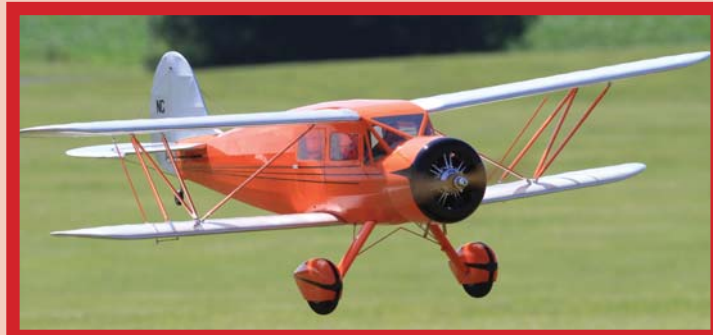
Adam Grubb assembled this Waco YKS-6 from a Pilot-1 ARF. The model has an O.S. 7-cylinder radial engine, which sounds great in the air!
