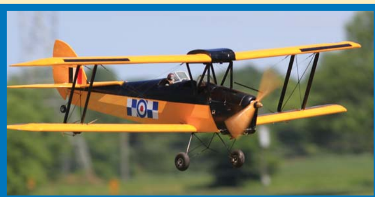
This kit-built de Havilland Tiger Moth, entered by Charles Gray, is powered by an O.S. .70 engine and uses a JR Colt radio system.
